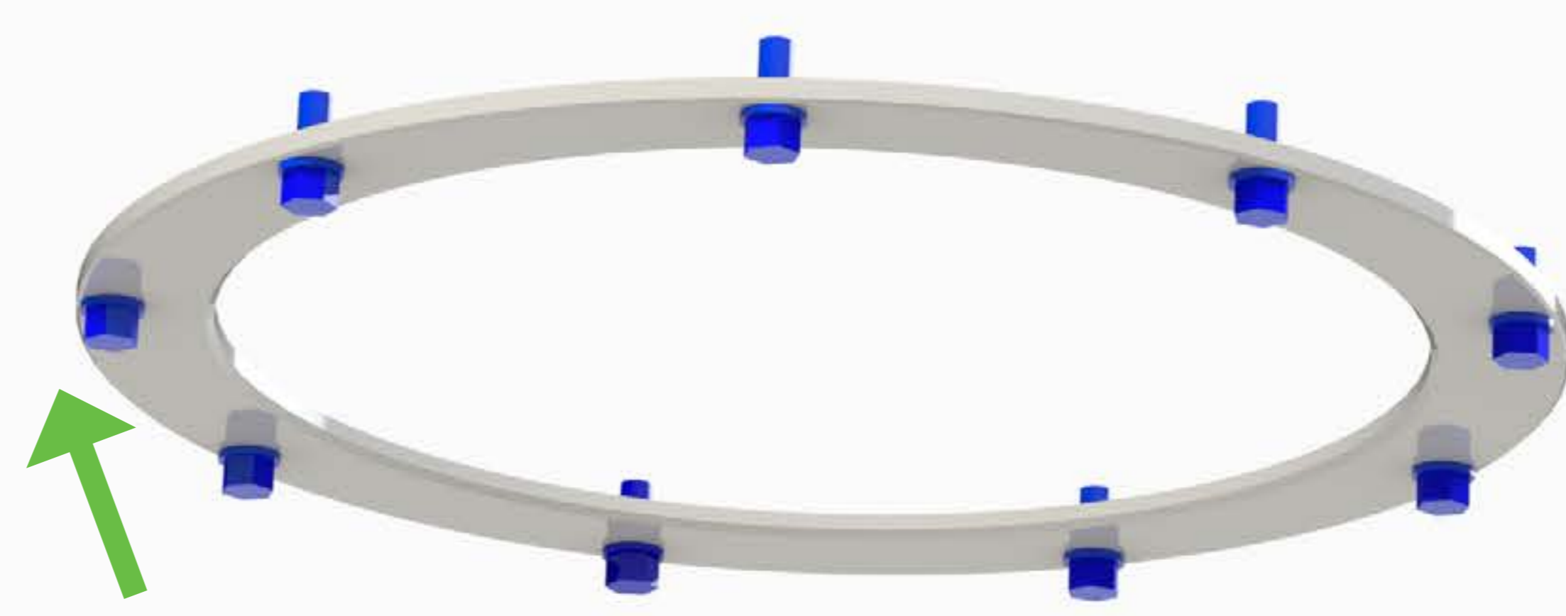
REMOVE LOWER RETAINER PLATE TO REMOVE SEAL
